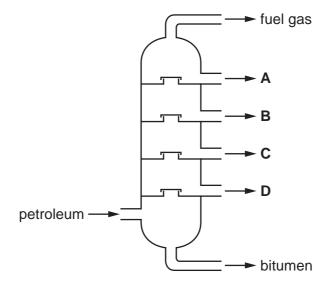
4 Petroleum is separated into fractions by fractional distillation.
